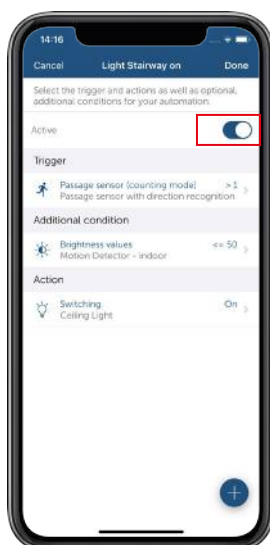
Figure 57: Activation and deactivation of automation
