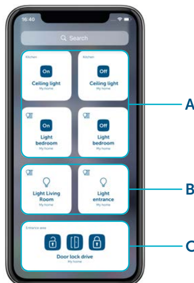
Figure 83: Screenshot – Homematic IP widgets: active and passive widgets
