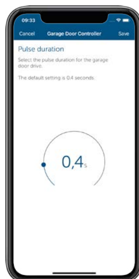
Figure 65: Screenshot garage door controller pulse duration
