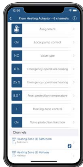
Figure 21: Screenshot device configuration Floor Heating Controller
