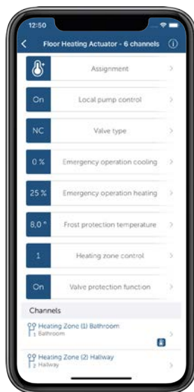
Figure 20: Screenshot device configuration Floor Heating Controller
