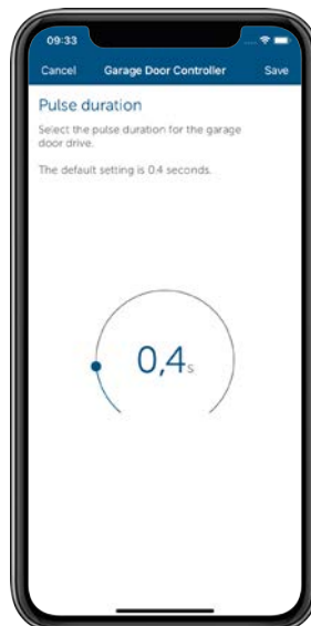
Figure 59: Screenshot garage door controller pulse duration
