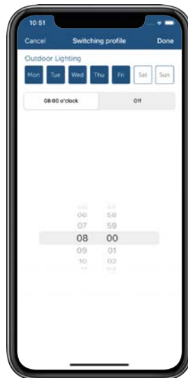
Figure 43: Screenshot Adjusting the switching profile
