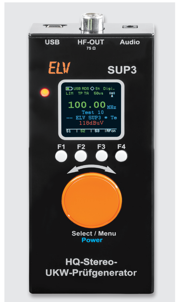
Figure 16: SUP3 Fully assembled and ready for operation
